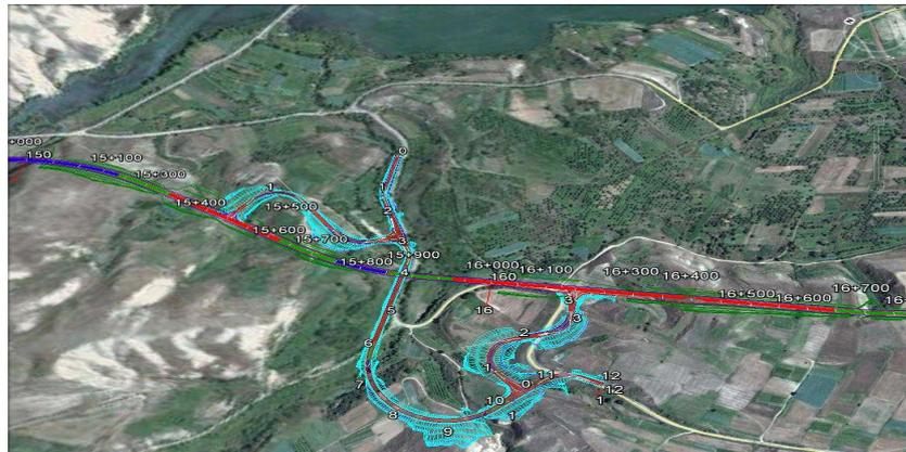
The interchange No. 3 is located approximately at km 57+500 and it is needed in order to re-establish the connection with the existing M2 road and to connect the new road with the East part of the Armenia such as Kapan, Syunik (shown in the following picture).
